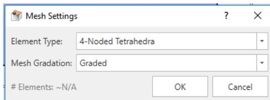
Enter Element Type = 4-Noded Tetrahedra, Mesh Gradation = Graded, [OK]. Then mesh the model: **Mesh → Mesh**. The model should appear as below:
