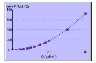
Figure 6. Pressure -Flow Piecewise Linear Correlation for Resistance Element
