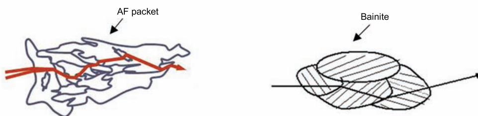
Fig. 5 Schematic illustration of acicular ferrite (AF) packet and bainite packet
