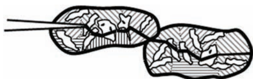
Fig. 7 Schematic illustration of the effect of acicular ferrite in bainite base on crack propagation
