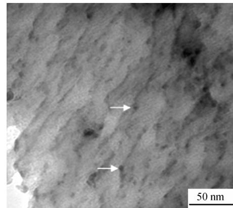
**Fig. 5.** TEM micrograph of precipitates in the specimen.
