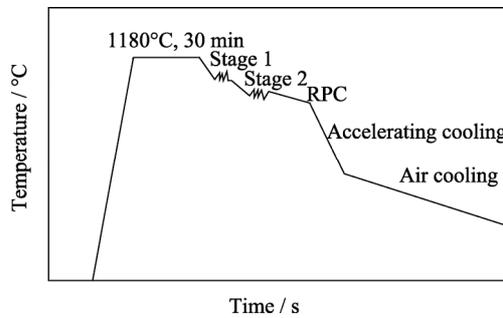
Fig. 1. Schematic illustration of an advanced TMCP-RPC process.
