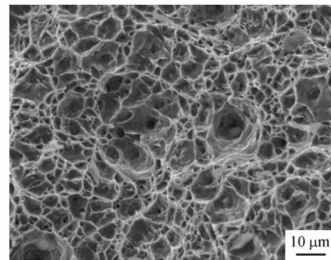
**Fig. 10.** SEM image of the tensile fracture specimen.
