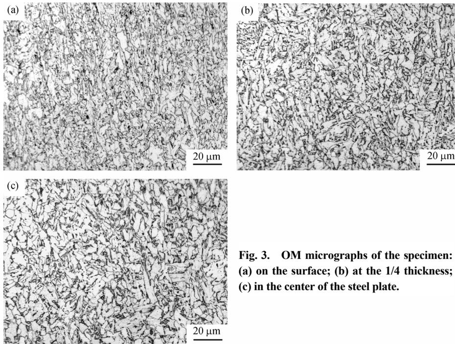
**Fig. 3.** OM micrographs of the specimen: (a) on the surface; (b) at the 1/4 thickness; (c) in the center of the steel plate.
