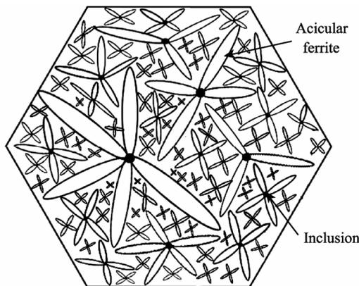
**Fig. 9.** Schematic illustration of the formation mechanism of interlocked acicular ferrite microstructures.
