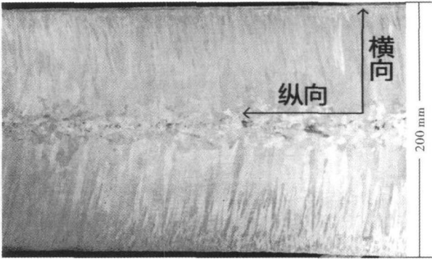
图 1 N08810 合金连铸板坯低倍组织及取样方向 Fig.1 Macrostructure and sampling direction of casting slab of N08810 alloy
