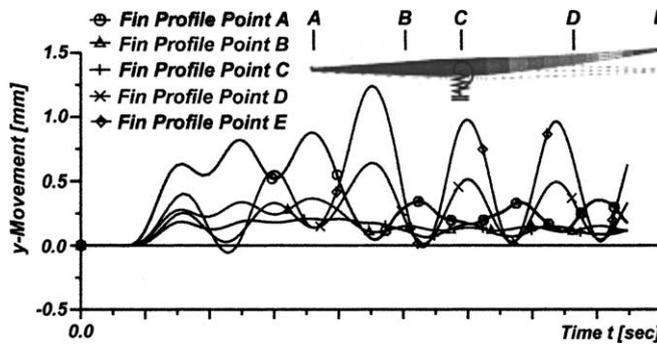
Fig. 10. Time history of fin profile structure movement due to flow conditions at Ma 2.0.
