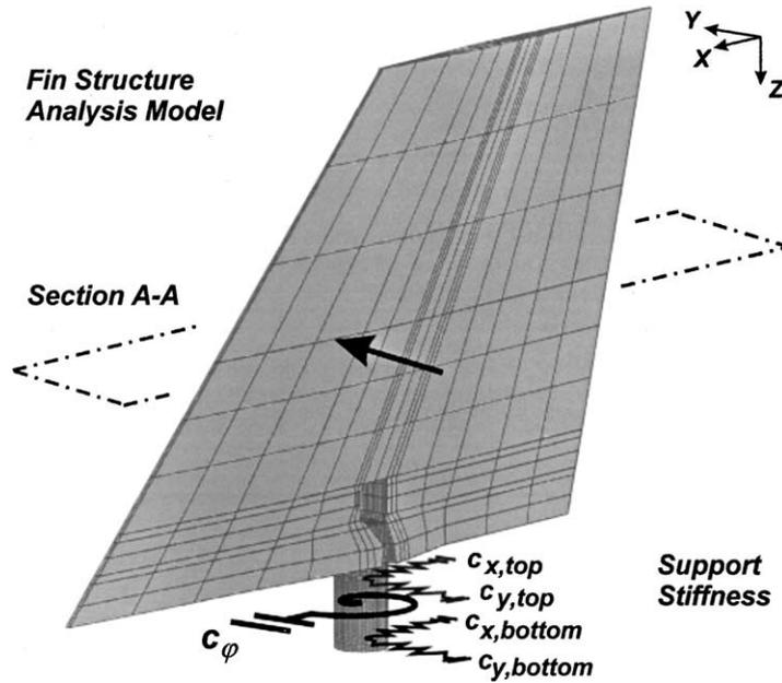
Fig. 1. Fin structure and boundary conditions (3D-model).
