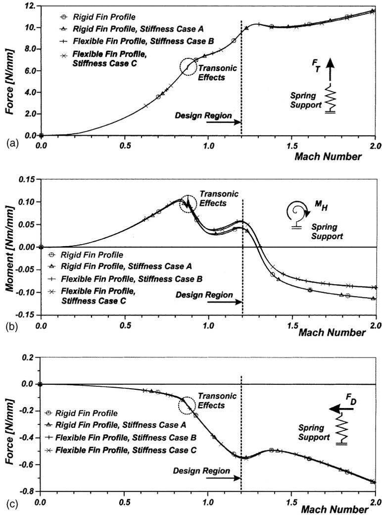
Fig. 6. (a) Translational spring force history due to unsteady aerodynamic pressure load, (b) spring moment history due to unsteady aerodynamic pressure load and (c) drag force history due to unsteady aerodynamic pressure load.
