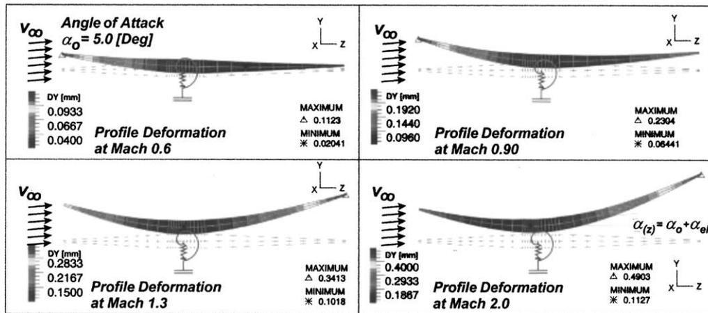
Fig. 8. Fin profile deformation, stiffness case C.
