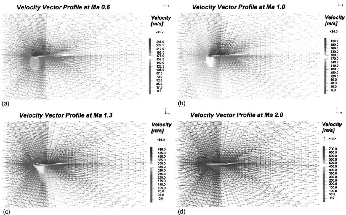
Fig. 4. (a–d) Velocity vector profiles up to Ma 2.0.
