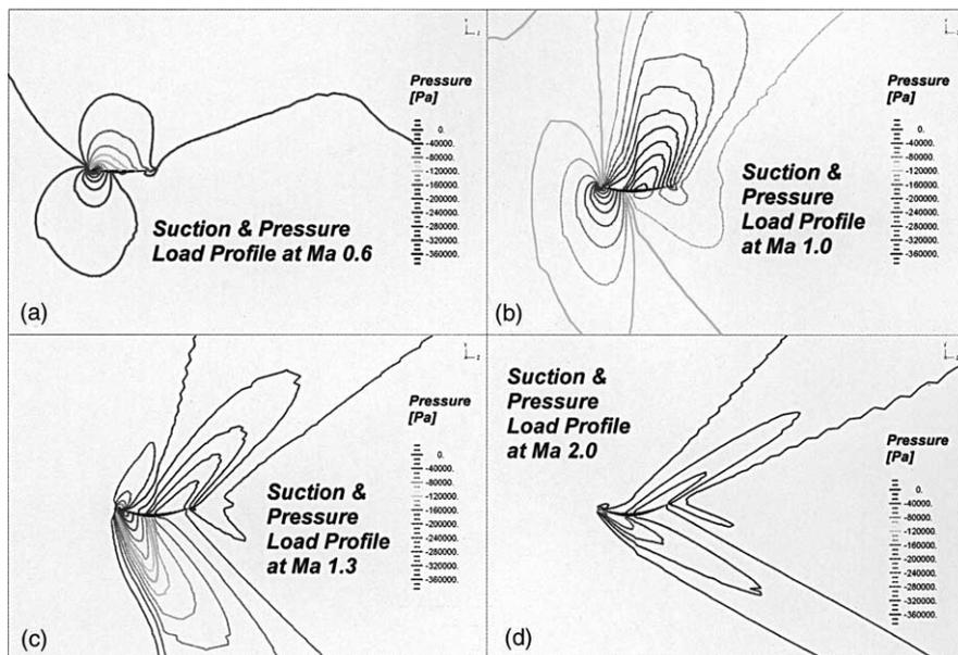
Fig. 5. (a–d) Suction and pressure load profiles on deformed fin profile structure up to Ma 2.0.
