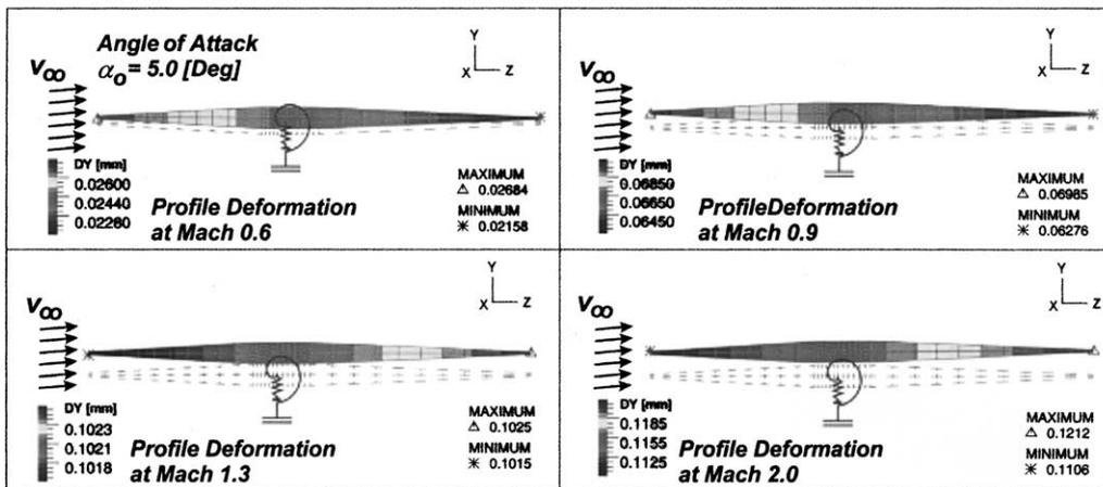
Fig. 7. Fin profile deformation, stiffness case A.
