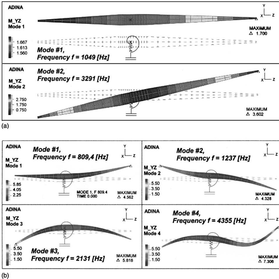
Fig. 3. (a) Frequency analysis—stiffness case A, mode shapes 1–2. (b) Frequency analysis—stiffness case B, mode shapes 1–4.
