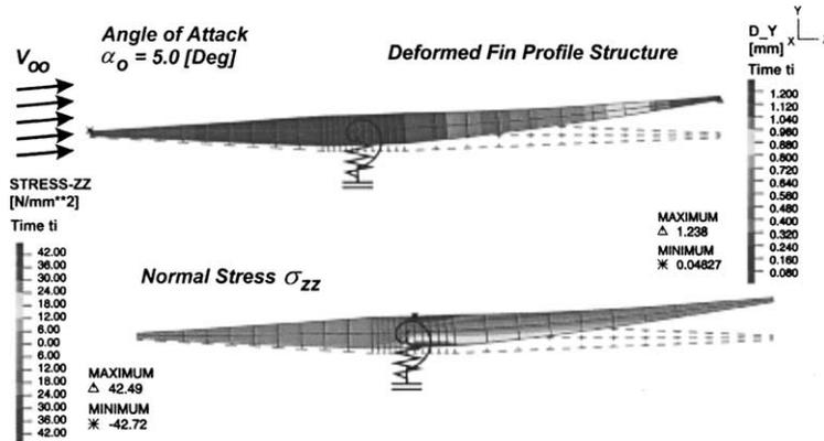
Fig. 9. Fin profile deformation and normal stresses at time  $t_i$  due to flow conditions at Ma 2.0.
