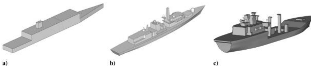
Fig. 4 CAD geometry of the ships used for the CFD airwake computations: a) SFS2, b) Type 23 frigate, and c) Wave class AO.
