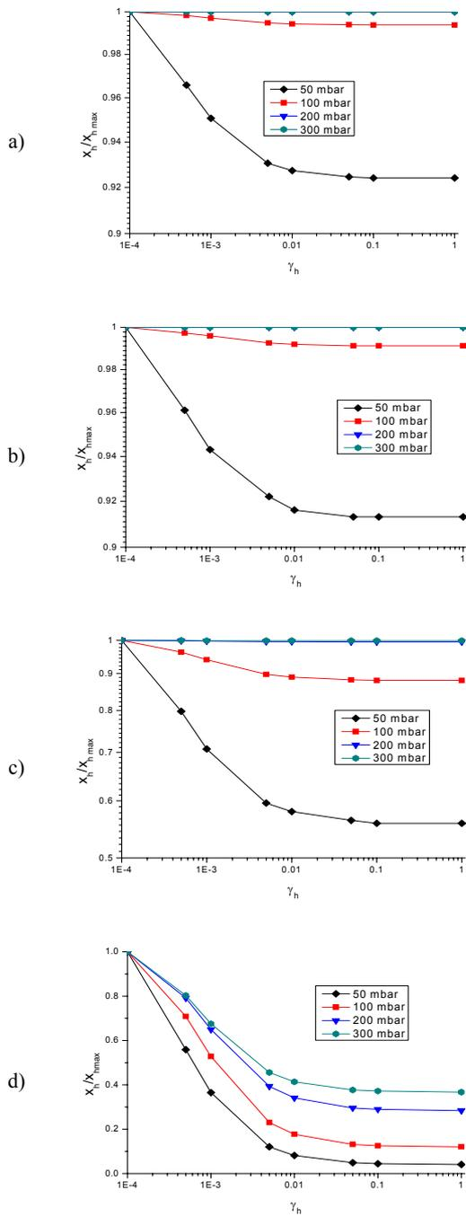
**Figure 4** : Atomic hydrogen mole fraction normalized by the maximum value, i.e.,  $\gamma_H=10^{-4}$ , **a)** in the plasma bulk., **b)** under the substrate holder in  $r=0$ , **c)** under the substrate holder at the right side, **d)** near the quartz wall.
