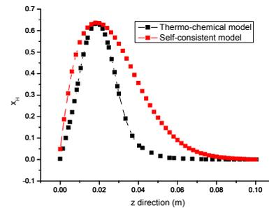
**Figure 9 :** Comparison of the axial distribution of atomic hydrogen for the thermo-chemical and self-consistent models.  $z=0$  correspond to the surface holder and  $z=0.1\text{m}$  to the quartz bell jar
