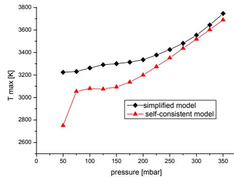
**Figure 3 :** Gas temperature obtained with simplified thermo-chemical model and with full self-consistent model ( $T_{\text{quartz}} = 400 \text{ K}$ ,  $\gamma_{\text{H}} = 0.1$ ).
