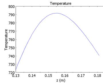
**Figure 6 :** Temperature on the quartz wall at 300 mbar. The maximum value is nearly located in the front of the hottest plasma point.
