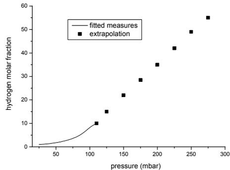
**Figure 2 :** Experimental results for hydrogen mole fraction in the plasma bulk as function of pressure (line: measured by optical spectroscopy; square: extrapolation of fitted data).
