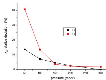
**Figure 7 :** deviation observed near the substrate holder (points B and C in Figure 1) in hydrogen mole fraction considering  $\gamma_H=0.1$  and  $\gamma_H$  following equation 5.
