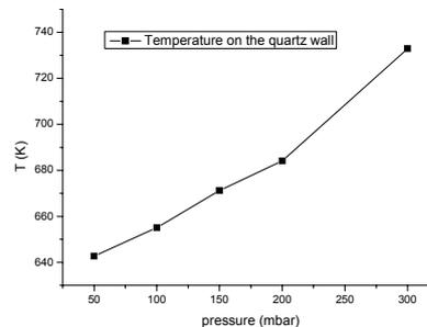
**Figure 8:** Temperature on the quartz wall of the Bell Jar reactor (at  $z_C = 0.132$  mm).
