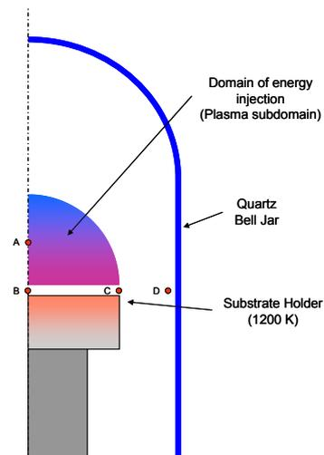
**Figure 1:** Computational domain of plasma Bell Jar reactor.
